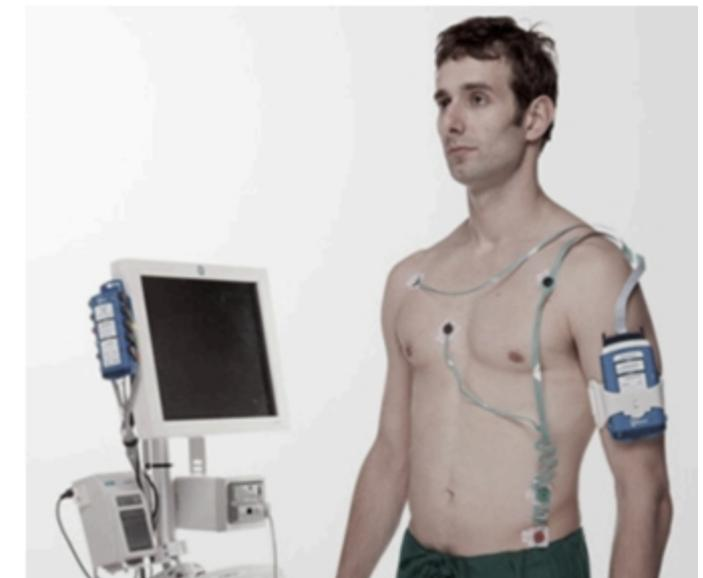
Fig 6. Low cost compact wireless ECG sensor. © Isansys Lifecare
