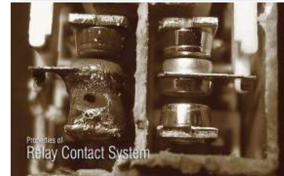
Pic1, lillie contact oxidation, fusion occurren
